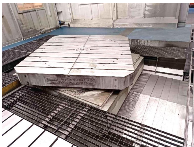
Mesa rototraslante vasculante motorizada \pm 5^\circ DEMMELER mod. DRALT2500 2500 x 2500 mm. / motorised rotary-translating Table with motorised tilt-table \pm 5^\circ DEMMELER mod DRALT2500. 2500 X 2500 mm.
